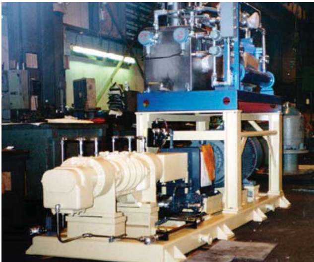
Figure 3 Twin-screw Naphtha Main Gas Turbine Fuel Pump
